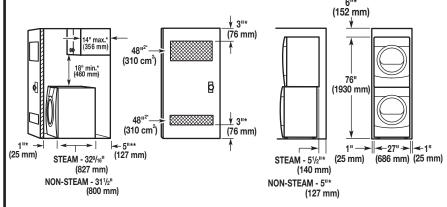
For cabinet installation, with a door, the minimum ventilation openings in the top are required.
